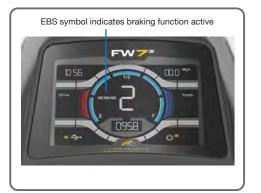
The FW7<sup>S</sup> EBS has the added advantage of an Electronic Braking System (EBS) for hill descent control.
