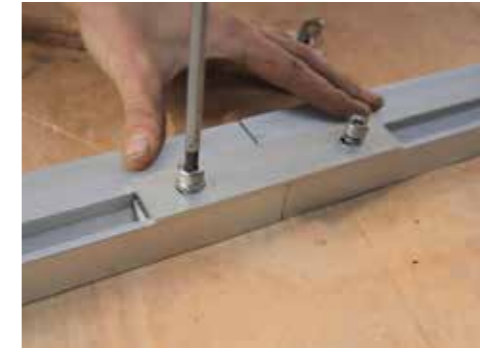
Tighten using a M6 Allen Key and use a torque wrench set at 15Nm to tighten
