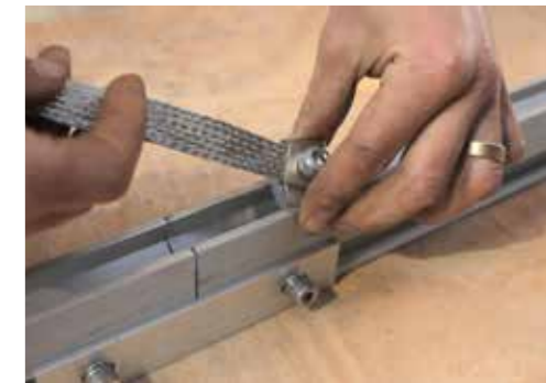
Wherever a Standard Rail Splice Kit is used a Bonding Jumper must also be attached to ensure a quality earth connection
