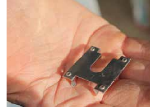
Grounding Clips are used to ensure the PV Panels are earth bonded to the mounting rail. The sharp edges of the Grounding Clips pierce the anodizing of the panel and rail to create the earth connection.
