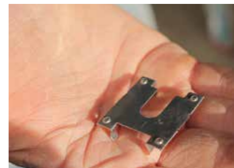
Grounding Clips are used to ensure the PV Panels are earth bonded to the mounting rail. The sharp edges of the Grounding Clips pierce the anodizing of the panel and rail to create the earth connection.
